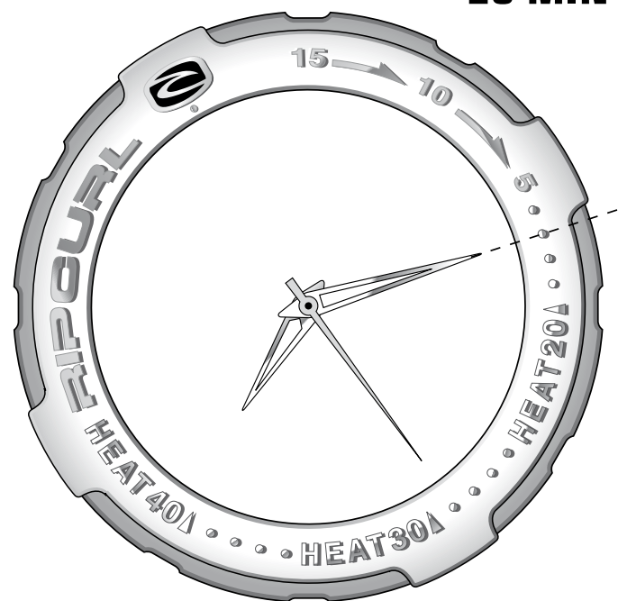
BEZEL INDICATING THREE MINUTES TO GO IN A 20 MIN HEAT
